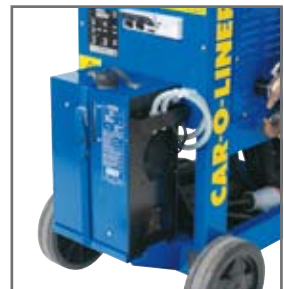
Water cooling unit
